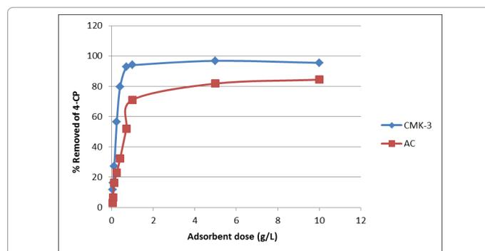
**Figure 6:** Adsorption isotherms (Removal %) of 4-Chlorophenol versus mesoporous and microporous carbons loading (4-CP concentration = 100 mg/L, agitation speed = 350 rpm, pH = 6, temperature = 25°C).
