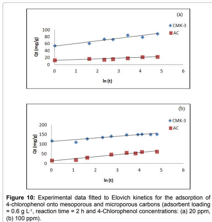
**Figure 10:** Experimental data fitted to Elovich kinetics for the adsorption of 4-chlorophenol onto mesoporous and microporous carbons (adsorbent loading = 0.6 g L<sup>-1</sup>, reaction time = 2 h and 4-Chlorophenol concentrations: (a) 20 ppm, (b) 100 ppm).
