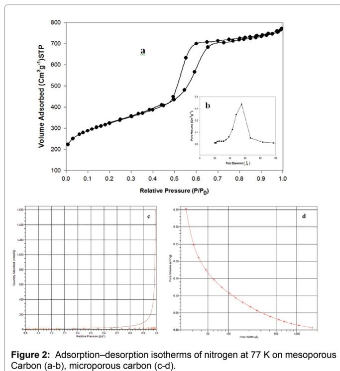
Figure 2: Adsorption-desorption isotherms of nitrogen at 77 K on mesoporous Carbon (a-b), microporous carbon (c-d).
