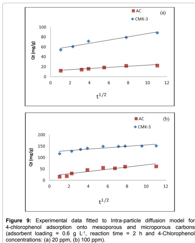
**Figure 9:** Experimental data fitted to Intra-particle diffusion model for 4-chlorophenol adsorption onto mesoporous and microporous carbons (adsorbent loading =  $0.6 \text{ g L}^{-1}$ , reaction time = 2 h and 4-Chlorophenol concentrations: (a) 20 ppm, (b) 100 ppm).
