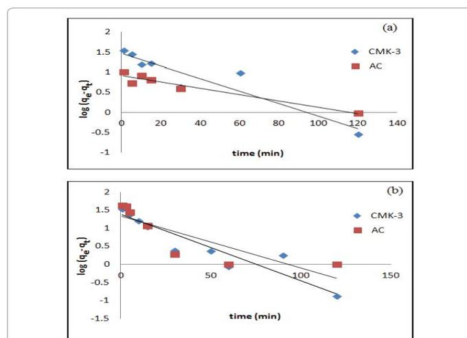
**Figure 7:** Experimental data fitted to Pseudo-first-order kinetics for the adsorption of 4-chlorophenol onto mesoporous and microporous carbons (adsorbent loading= 0.6 g L<sup>-1</sup>, reaction time = 2 h and 4-Chlorophenol concentrations: (a) 20 ppm, (b) 100 ppm).
