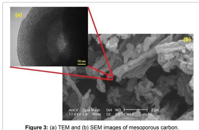
Figure 3: (a) TEM and (b) SEM images of mesoporous carbon.
