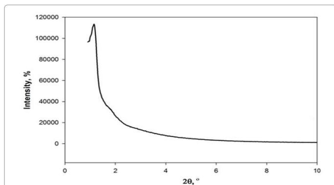
Figure 1: Low-angle X-ray diffraction pattern of ordered mesoporous carbon.
