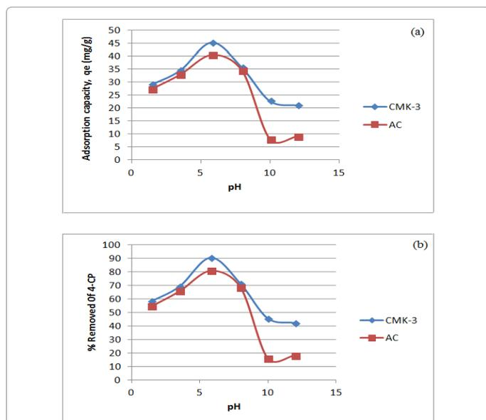
**Figure 4:** Effect of pH on the adsorption capacity of 4-Chlorophenol over mesoporous and microporous carbons (a) and its removal percent (b) (Adsorbent loading = 0.5 g/L, 4-CP concentration = 100 ppm, agitation speed = 350 rpm, temperature = 25°C).
