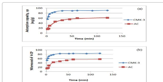
**Figure 5:** Effect of reaction time on the adsorption capacity of 4-Chlorophenol over mesoporous and microporous carbons (a) and its removal percent (b) (4-CP concentration = 100 ppm, adsorbent loading = 0.3 g/L, pH = 6, agitation speed = 350 rpm, temperature = 25°C).
