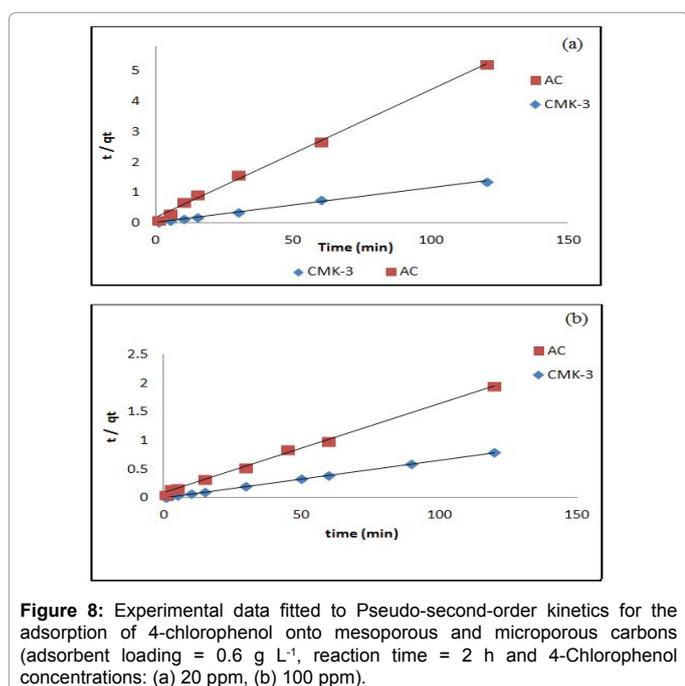
**Figure 8:** Experimental data fitted to Pseudo-second-order kinetics for the adsorption of 4-chlorophenol onto mesoporous and microporous carbons (adsorbent loading =  $0.6 \text{ g L}^{-1}$ , reaction time = 2 h and 4-Chlorophenol concentrations: (a) 20 ppm, (b) 100 ppm).
