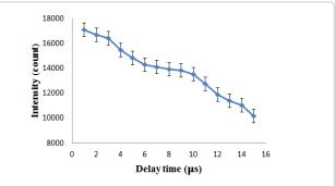
Figure 6: A plot of the characteristic intensities of the Mg spectra versus the delay time, with laser energy of 500 mJ and a pulse repetition rate of 1 Hz.
