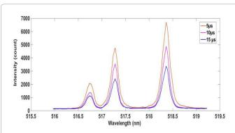
Figure 3: Time-resolved emission spectra of a laser-induced Mg plasma at a delay time of 5  $\mu$ s, 10  $\mu$ s and 15  $\mu$ s, in the spectral region of 515.97-519.22 nm.
