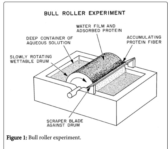
Figure 1: Bull roller experiment.
