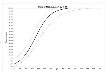
**Figure 2:** Risk of concussion among 312 non-duplicated helmeted players, by Head Injury Criterion (HIC). The dashed line indicates the 95% confidence interval for the risk curve.
