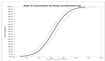
**Figure 1:** Risk of concussion among 312 non-duplicated helmeted players, by linear acceleration (g). The dashed line indicates the 95% confidence interval for the risk curve.
