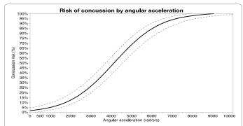
**Figure 3:** Risk of concussion among 312 non-duplicated helmeted players, by angular acceleration (rad/s²). The dashed line indicates the 95% confidence interval for the risk curve.
