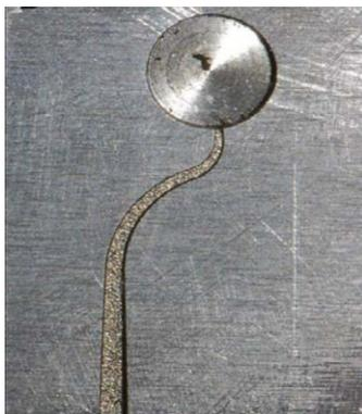
Figure 1: Artificial double curvature root canal used to test cyclic fatigue.
