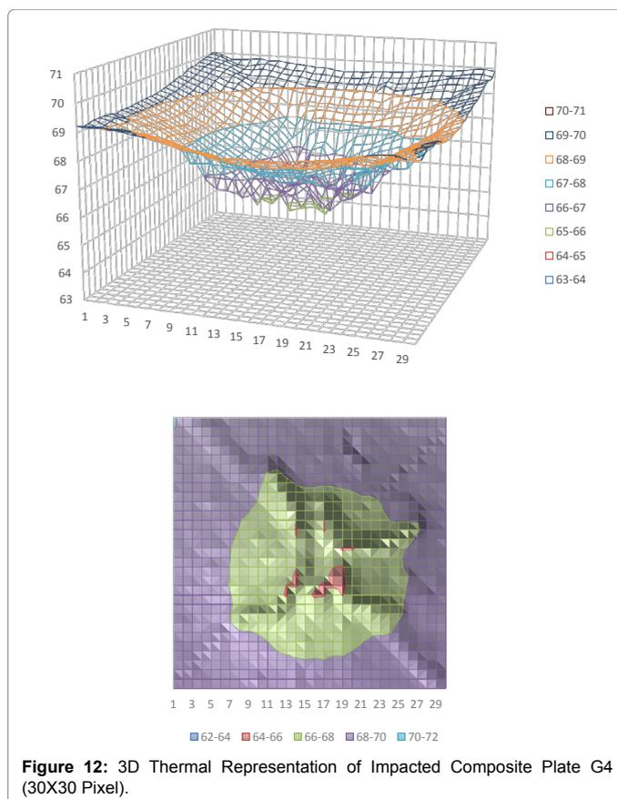
Figure 12: 3D Thermal Representation of Impacted Composite Plate G4 (30X30 Pixel).
