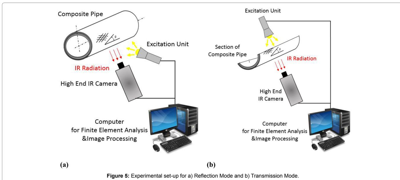
Figure 5: Experimental set-up for a) Reflection Mode and b) Transmission Mode.
