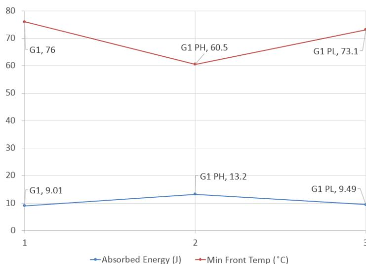
Figure 10: Absorbed energy vs. Minimum thermography Temperature for Glass Sample No.1 with different resin types.
