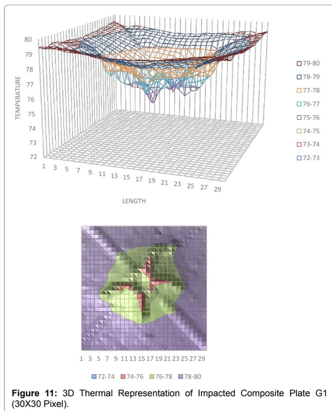
Figure 11: 3D Thermal Representation of Impacted Composite Plate G1 (30X30 Pixel).
