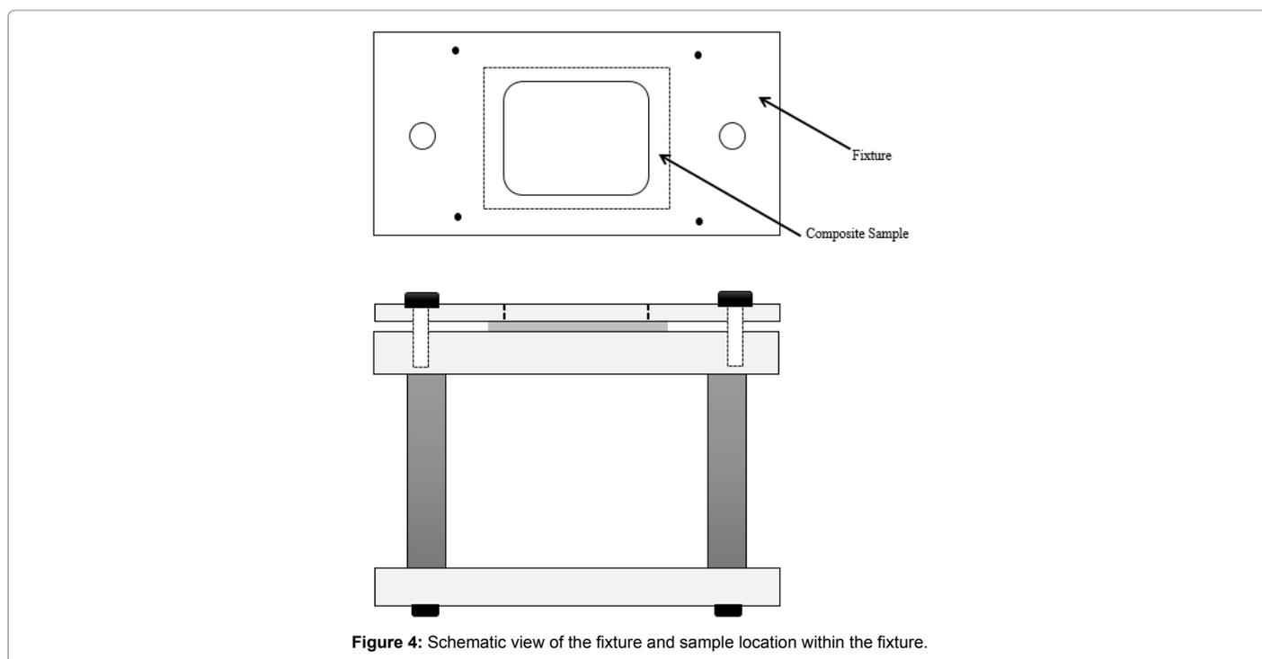
The composite plates were clamped along all edges. Clamping force is provided by steel plates on the top and bottom edges as shown in the schematic drawing (Figure 4). The clamping force is applied by tightening 2 bolts at edge of the fixture.
