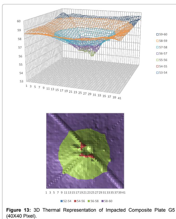
Figure 13: 3D Thermal Representation of Impacted Composite Plate G5 (40X40 Pixel).
