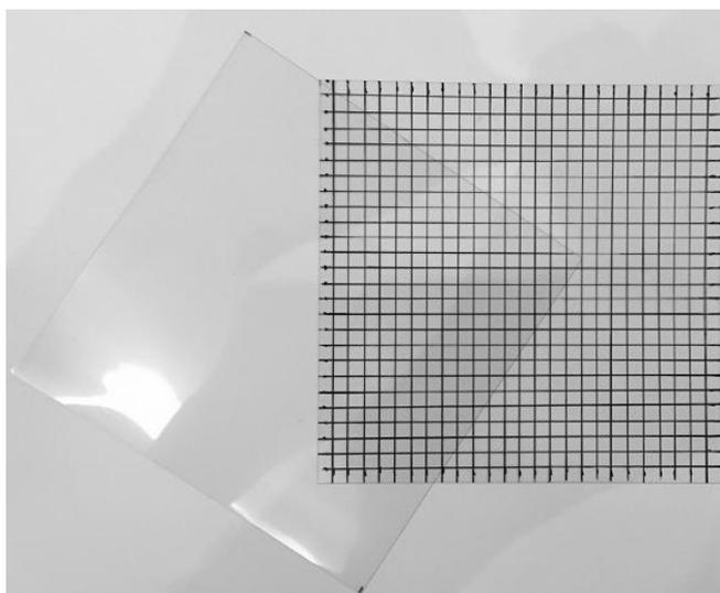
Figure 7: Transparent paper used for damage measurement.
