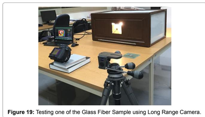
this study, lock-in thermography with advanced mid-wave camera and image processing produce were adopted to get better results in this study. To prove the above mentioned conclusion, same test was conducted for G4, G5, C1 and C4 plate's samples using long-wave thermal imaging camera (FLIR T650sc [24]) as shown in Figure 19) and the results were not satisfactory as there was no clear images captured after exposing the samples for 10 minutes heat as can be seen in Table 7.
