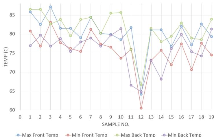
Figure 9: Measured Temperatures using Active Thermography where minimum values were observed at damage locations.
