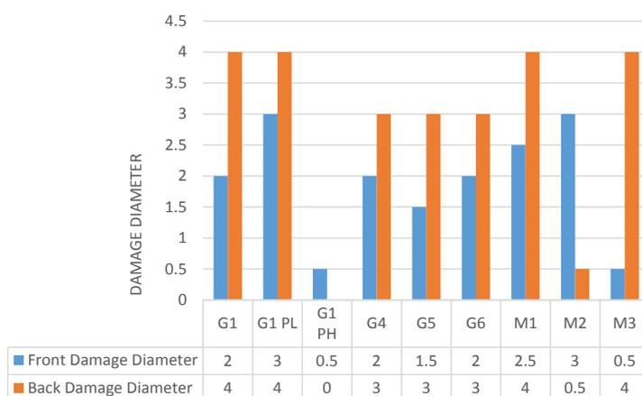
Figure 8: Summary of the damage measurement for glass and mixed fiber samples.
