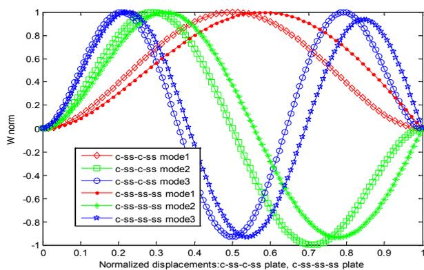
Figure 5: Normalized displacements for clamped and simply supported plates, for  $a/b=0.025$ ;  $h=0.03$ ,  $D_k=0.0$ ,  $E_f=0.0$ .
