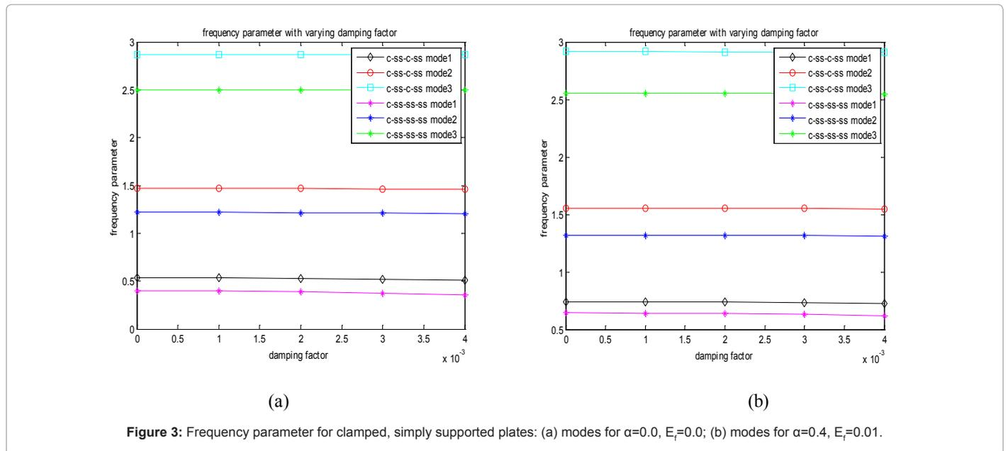
Figure 3: Frequency parameter for clamped, simply supported plates: (a) modes for  $\alpha=0.0, E_f=0.0$ ; (b) modes for  $\alpha=0.4, E_f=0.01$ .
