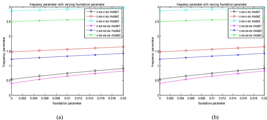
Figure 4: Frequency parameter for clamped, simply supported plates: (a) modes for  $\alpha=0.04$ ,  $D_k=0.0$ ; (b) modes for  $\alpha=0.4$ ,  $D_k=0.0025$ .
