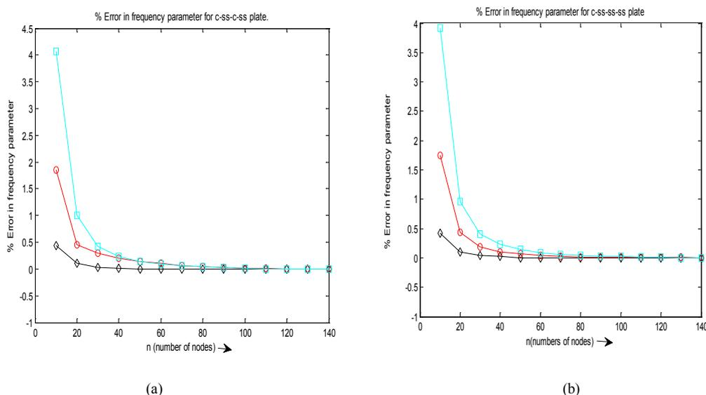
Figure 1: percentage error in frequency parameter  $\Omega$ : (a) c-ss-c-ss plate (b) c-ss-ss-ss plate, for  $a/b=0.25$ ,  $\alpha=0.0$ ,  $D_k=0.0$ , Percentage error= $[(\Omega_n - \Omega_{140}) / \Omega_{140}] \times 100$ ;  $n=10(10)140$ .
