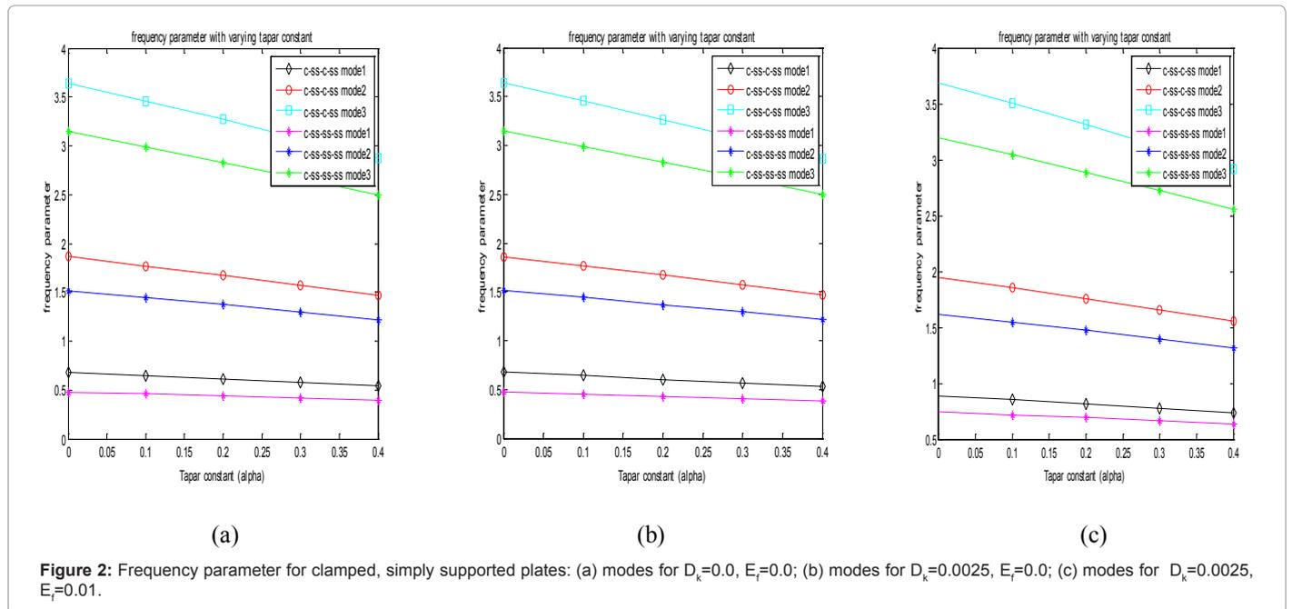
Figure 2: Frequency parameter for clamped, simply supported plates: (a) modes for  $D_k=0.0, E_f=0.0$ ; (b) modes for  $D_k=0.0025, E_f=0.0$ ; (c) modes for  $D_k=0.0025, E_f=0.01$ .
