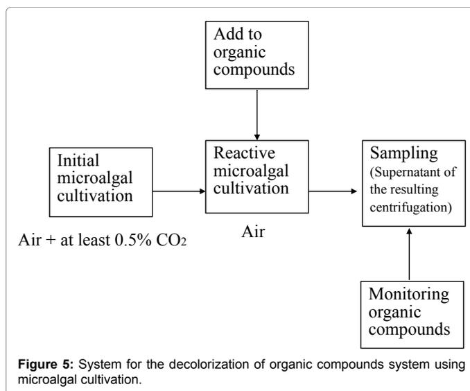
Figure 5: System for the decolorization of organic compounds system using microalgal cultivation.
