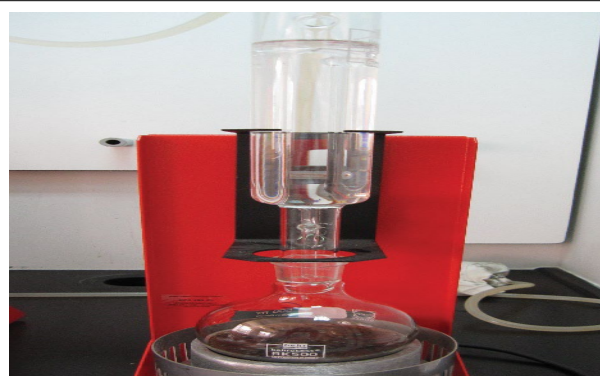
Figure 2: Soxhlet distillation set-up of asphaltene sample.
