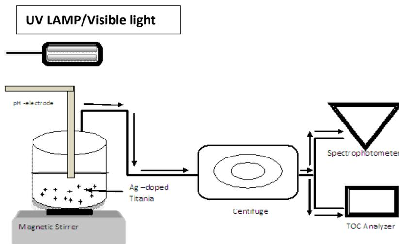
**Figure 2:** Experimental Setup for Photocatalysis under UV light/ Visible light
