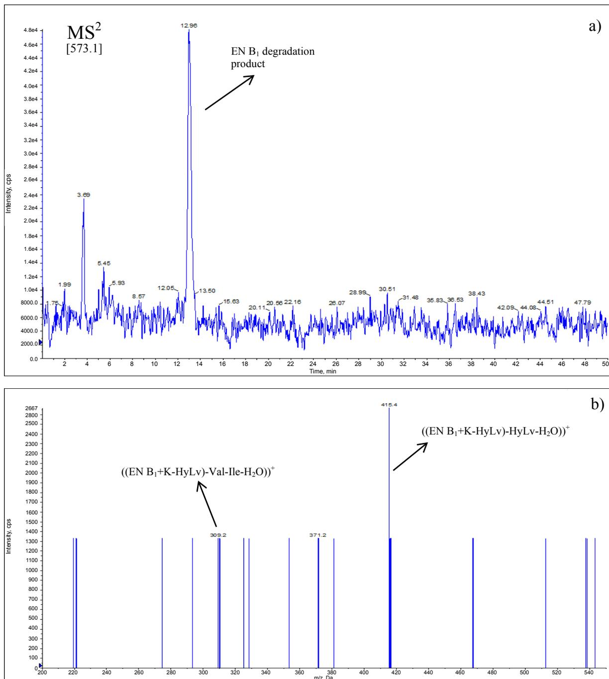
**Figure 6:** Chromatogram obtained in EPI mode (MS<sup>2</sup>) using as fragmenting ion the signal with an m/z of 573.10 of the EN B<sub>1</sub> degradation product a) and EPI mass spectrum b).
