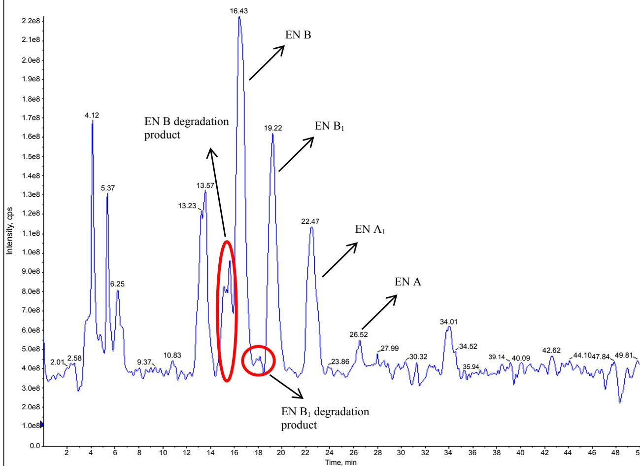
Figure 3: LC-MS-LIT chromatogram in ER mode of the ENs and its degradation products present in TSB medium after the fermentation by the strain of *Bacillus subtilis* CECT 4522.
