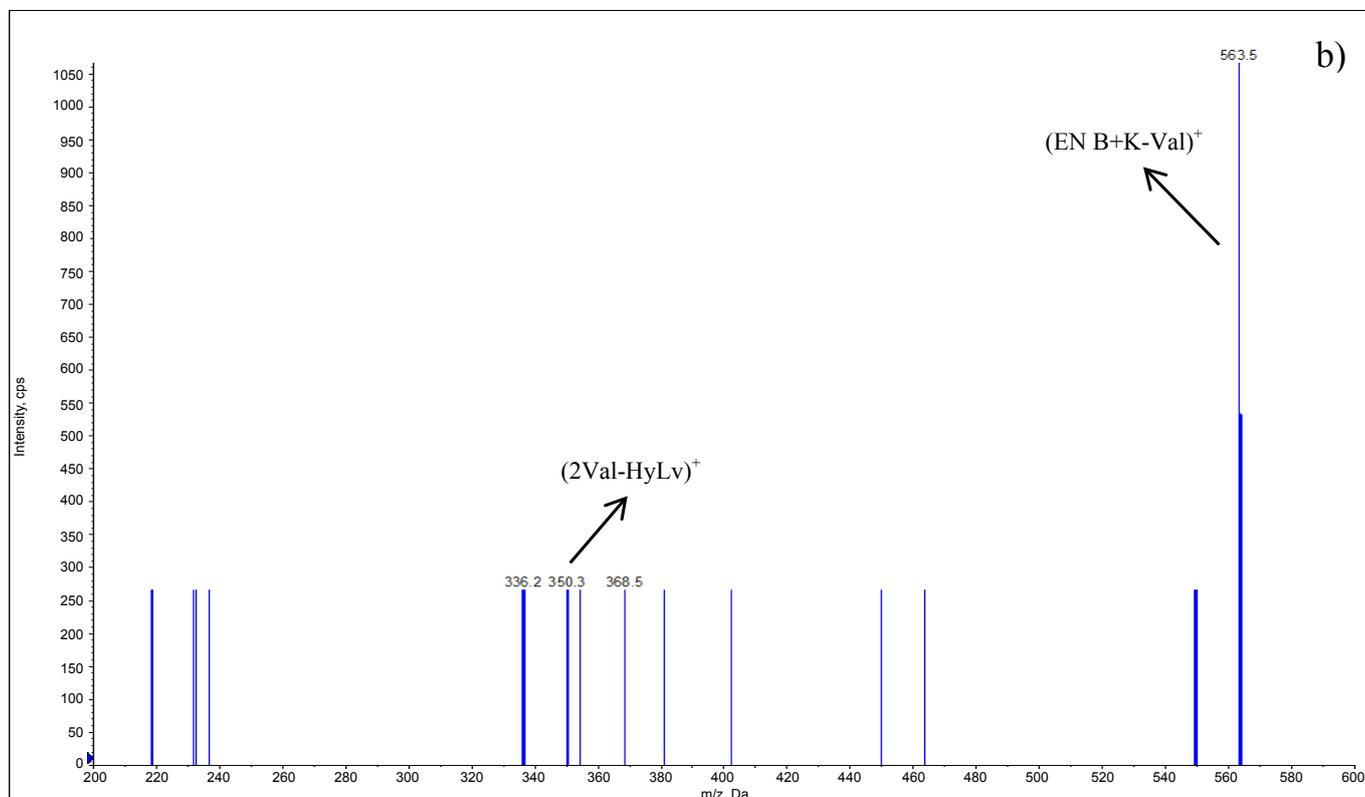
Figure 5: Chromatogram obtained in EPI mode (MS<sup>2</sup>) using as fragmenting ion the signal with a *m/z* of 561.2 of the EN B degradation product a) and EPI mass spectrum b).
