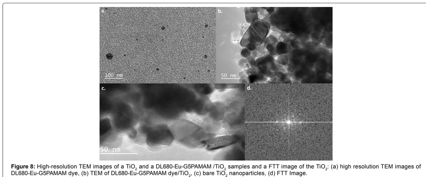
Figure 8: High-resolution TEM images of a TiO<sub>2</sub> and a DL680-Eu-G5PAMAM /TiO<sub>2</sub> samples and a FTT image of the TiO<sub>2</sub>: (a) high resolution TEM images of DL680-Eu-G5PAMAM dye, (b) TEM of DL680-Eu-G5PAMAM dye/TiO<sub>2</sub>, (c) bare TiO<sub>2</sub> nanoparticles, (d) FTT Image.
