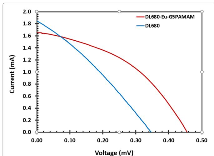
Figure 10: Photocurrent-voltage characteristics of DL680 and DL680-Eu-G5PAMAM dye sensitized solar cell measured under illumination of 100 mW/cm<sup>2</sup> (1.5 AM).
