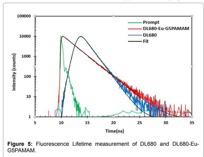
Figure 5: Fluorescence Lifetime measurement of DL680 and DL680-Eu-G5PAMAM.
