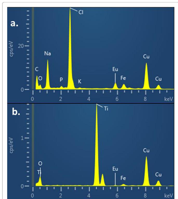
Figure 9: EDS Analysis of DL680-Eu-G5PAMAM without TiO<sub>2</sub> nanoparticles (a) and with TiO<sub>2</sub> nanoparticles (b).
