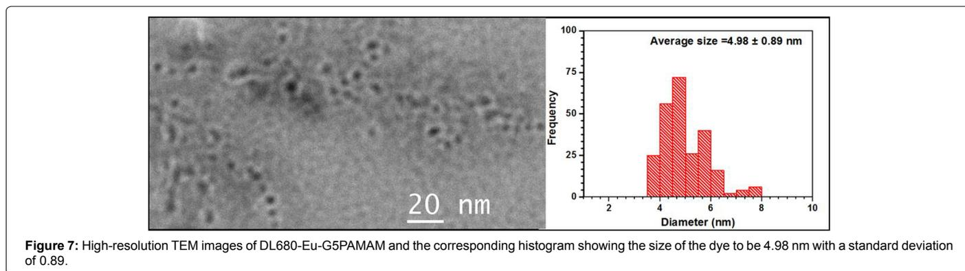
Figure 7: High-resolution TEM images of DL680-Eu-G5PAMAM and the corresponding histogram showing the size of the dye to be 4.98 nm with a standard deviation of 0.89.
