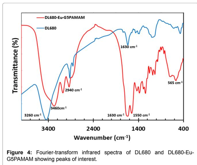
Figure 4: Fourier-transform infrared spectra of DL680 and DL680-Eu-G5PAMAM showing peaks of interest.
