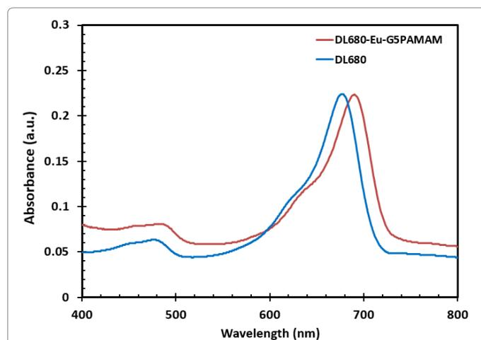
Figure 2: Absorption spectra of aqueous solutions of DL680 and DL680-Eu-G5PAMAM dyes.
