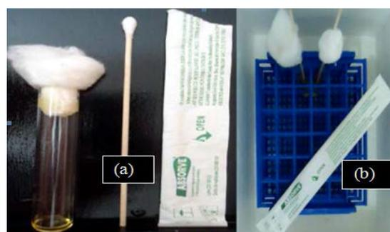
Figure 1: Test tube with BHI and sterile swab with wooden rod (a) and Styrofoam box with test tubes (b) used in data collection.
