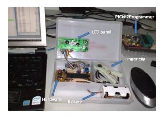
Figure 1: Experimental set-up of pulse oximeter
