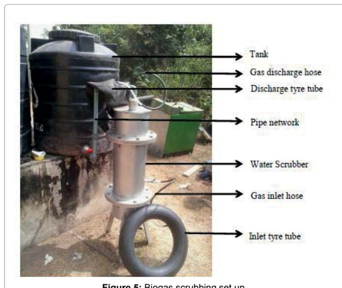
Figure 5: Biogas scrubbing set up.
