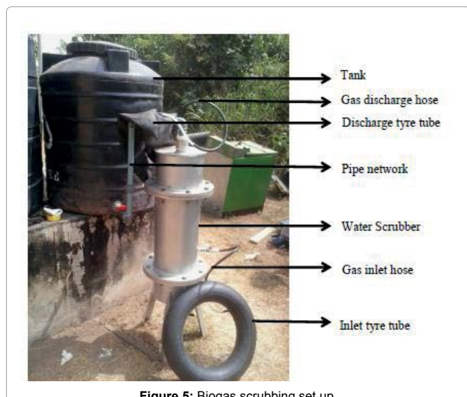
Figure 5: Biogas scrubbing set up.
