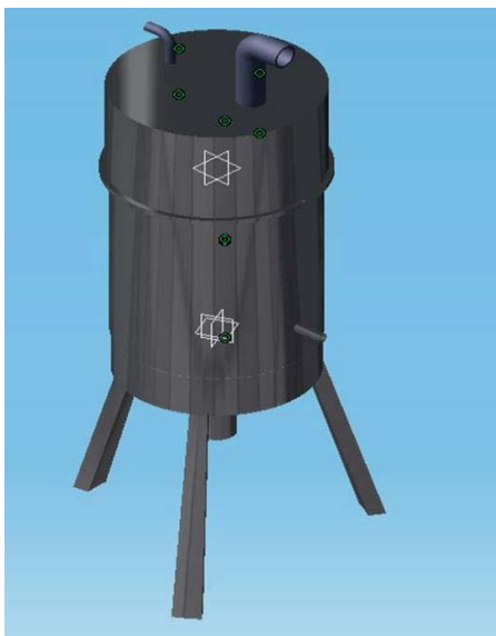
Figure 1: Isometric view of the Water scrubber with an iron wool packed bed.
