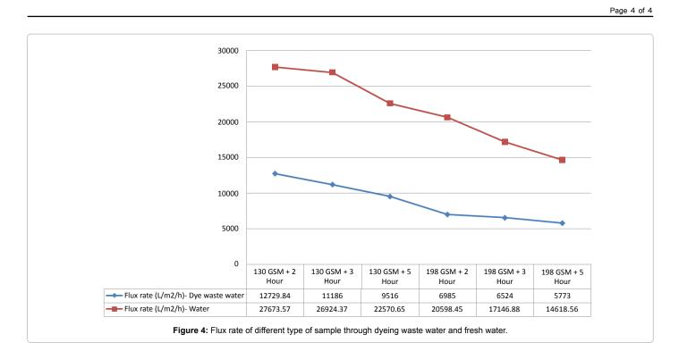
the Microfiltration cleaning efficiency is 70%. So, by using this type of composite nonwoven for pre-filtration of microfiltration process, cleaning efficiency around 91% can be achieved. Achieving this much high cleaning efficiency, improves the efficiency of further cleaning process.
