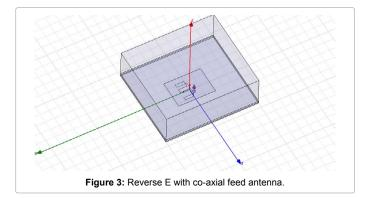
7.45-8.15 GHz with -20 dB gain and 8.8-9.2 GHz with -17 dB gain and this frequencies has the following applications.
