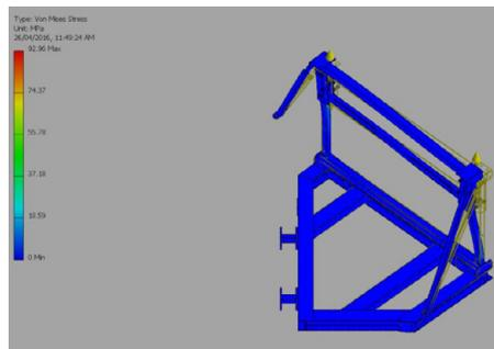
Figure 6: Maximum stress in belt entry/exit roller frames.
