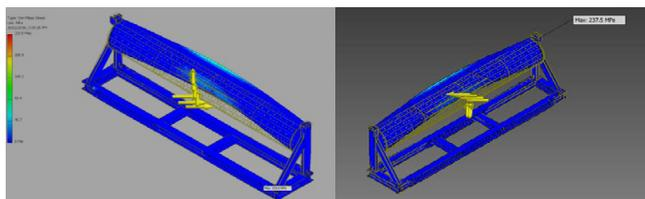
Figure 4: Maximum Stress in Turning Frame from 1000 mm wide belt (L) and from 2000 mm wide belt (R).
