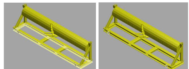
**Figure 2:** Turning Frame supported by level ground (L) Turning Frame fixed points(R).
