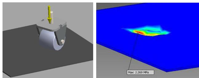
Figure 7: Force applied on roller to belt (L) Maximum stress on belt from one roller (R).
