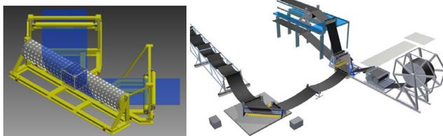
**Figure 1:** Overview of 10T 90° Turning frame showing rollers and belt (L) Typical belt installation at site showing use of Turning Frames 2 (R).
