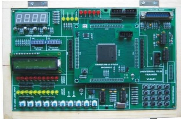
Figure 8: Snap shot of Spartan-3 FPGA Kit
