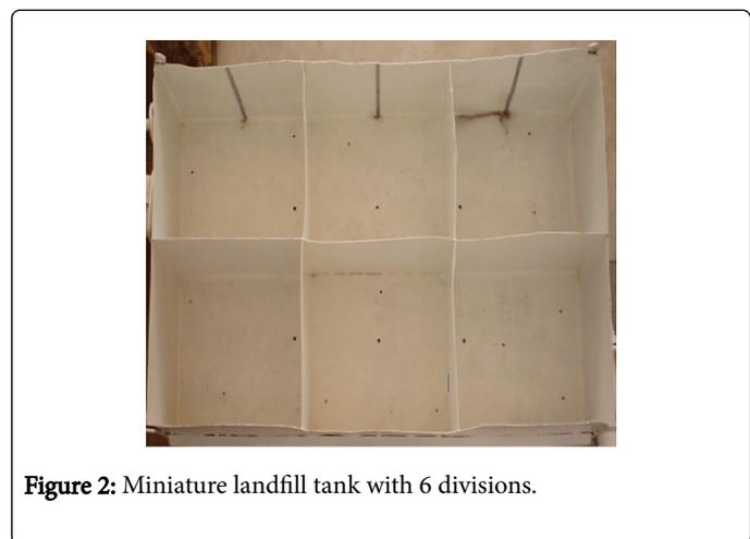
**Figure 2:** Miniature landfill tank with 6 divisions.
