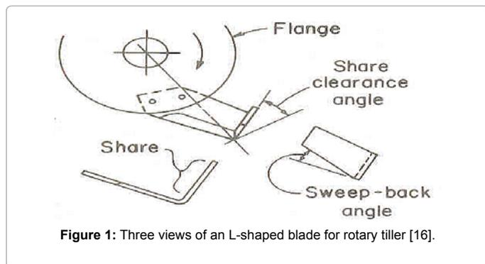
Figure 1: Three views of an L-shaped blade for rotary tiller [16].
