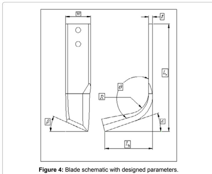
Figure 4: Blade schematic with designed parameters.
