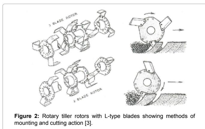
Figure 2: Rotary tiller rotors with L-type blades showing methods of mounting and cutting action [3].
