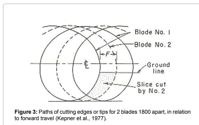
Figure 3: Paths of cutting edges or tips for 2 blades 180° apart, in relation to forward travel (Kepner et al., 1977).
