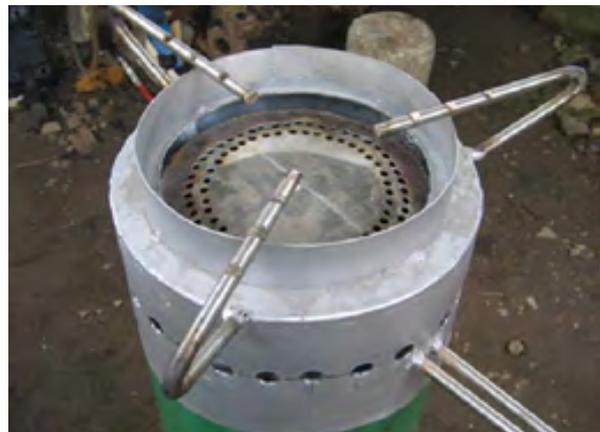
**Figure 5:** The Gas Burner consists a pot support and a burner with holes of diameter 3-4 mm.
