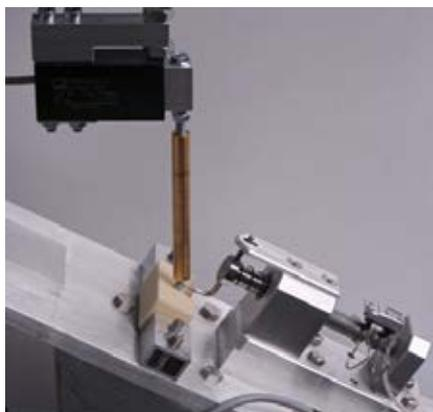
**Figure 3:** Specimen consisting of an implant placed in bone surrogate material placed in a universal testing machine at an angle of 30° with respect to the long axis of the implant. Load is applied through the brass-colored bar while implant displacement is transferred to a remotely positioned extensometer.
