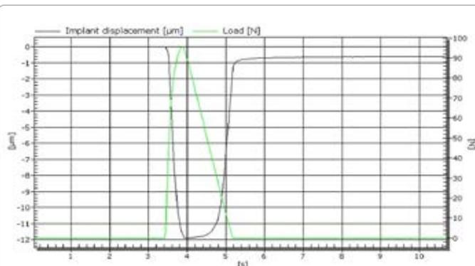
**Figure 4:** Screenshot from the analyzing software displaying load application and resulting implant displacement over time.
