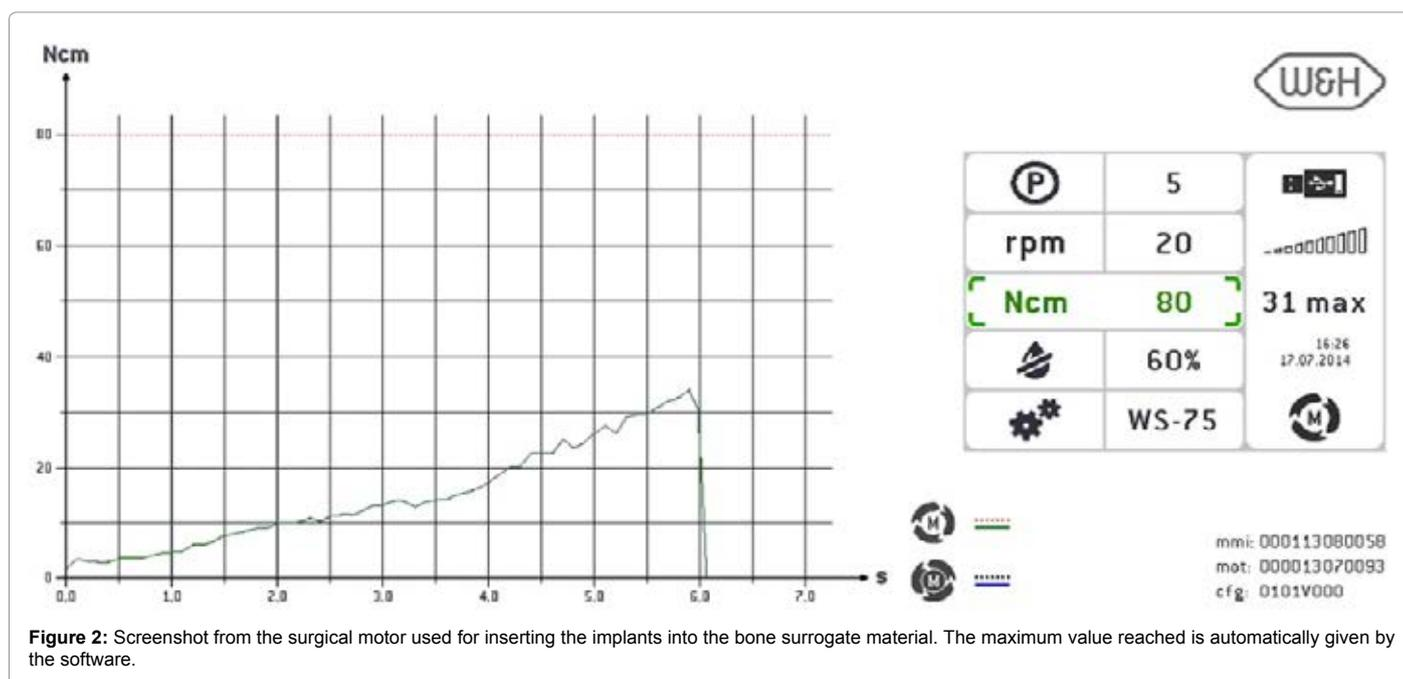
**Figure 2:** Screenshot from the surgical motor used for inserting the implants into the bone surrogate material. The maximum value reached is automatically given by the software.
