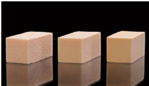
**Figure 1b:** Bone surrogate materials used in this study showing a homogeneous, solid structure and densities of 10 pcf, 20 pcf and 30 pcf (from left to right).
