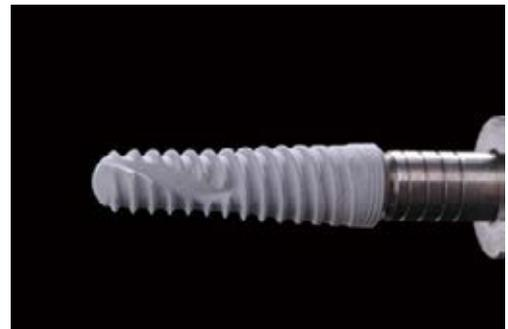
**Figure 1a:** Bone level dental implants used in this study which were inserted into bone surrogate materials leaving 3 mm of the implant extending from the surface of the bone blocks.
