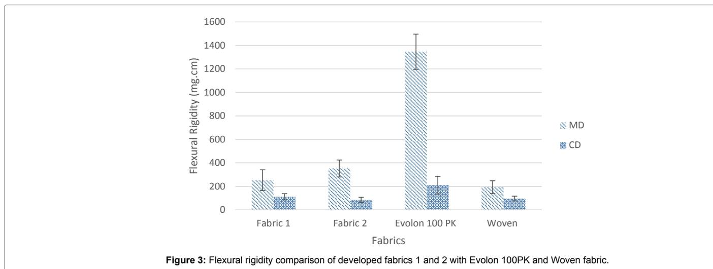
Figure 3: Flexural rigidity comparison of developed fabrics 1 and 2 with Evolon 100PK and Woven fabric.
