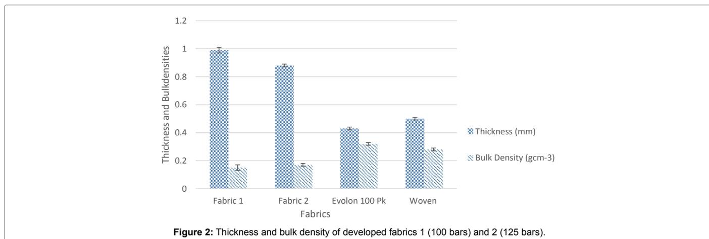
Figure 2: Thickness and bulk density of developed fabrics 1 (100 bars) and 2 (125 bars).
