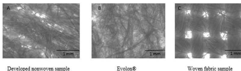
Figure 4: Microscopic Views of (a) developed hydroentangled, (b) Evolon® and (c) woven.
