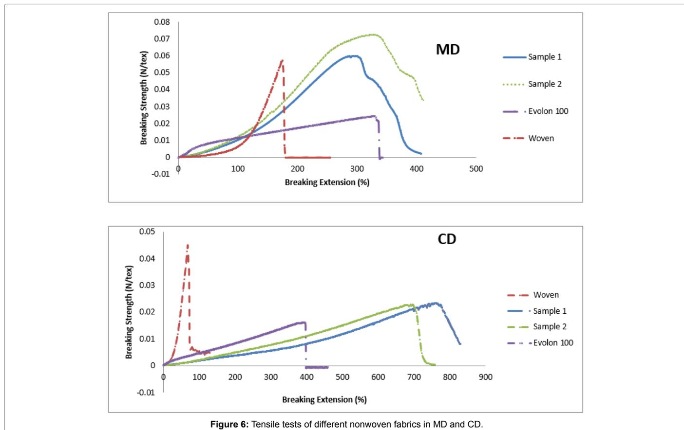
Figure 6: Tensile tests of different nonwoven fabrics in MD and CD.
