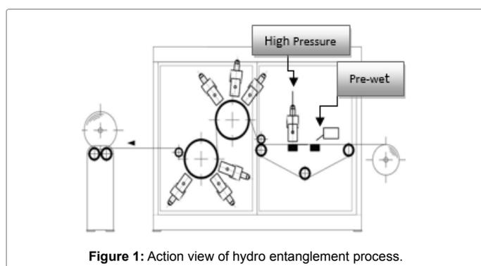
Figure 1: Action view of hydro entanglement process.
