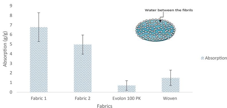
Figure 5: Absorption properties of nonwoven fabrics.
