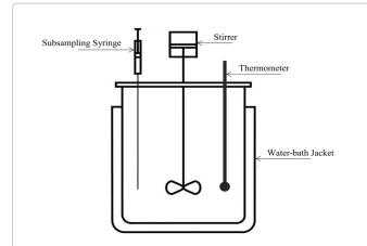
**Figure 1:** Experimental setup for the lipolysis of olive oil emulsion. Water jacket is used to control reaction temperature. Stirrer impeller is used to mix the emulsion substrate during the reaction. In a pre-adjusted periods, sub-sampler syringe is used to collect the samples.
