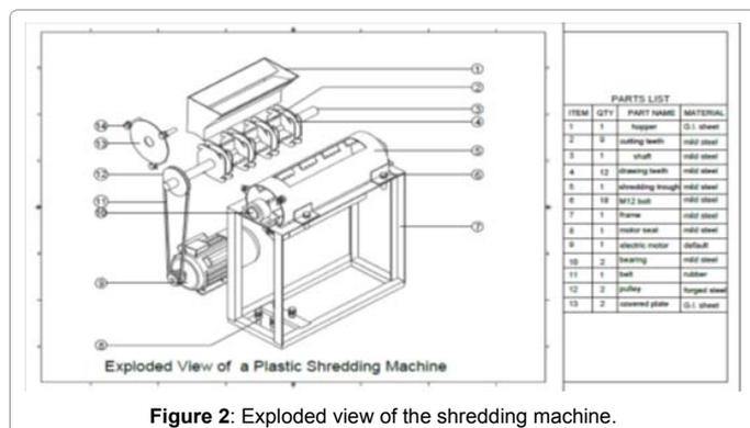
Figure 2: Exploded view of the shredding machine.
