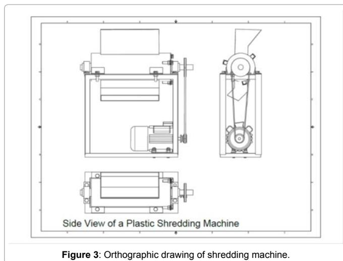
Figure 3: Orthographic drawing of shredding machine.
