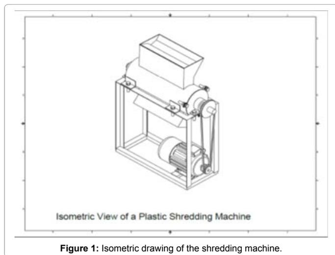
Figure 1: Isometric drawing of the shredding machine.
