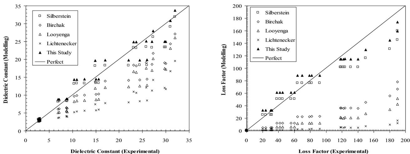
Figure 7: comparison of experimental and theoretical dielectric constant and loss factor of diesel contaminated soil.
