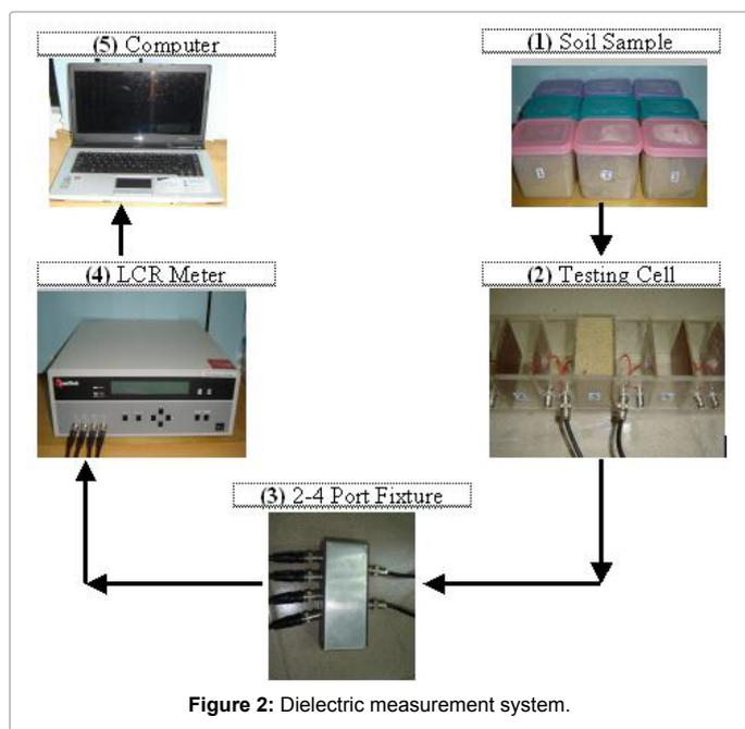
calculated and a PC logs all data. The complex permittivities (real part dielectric constant and imaginary part loss factor) of soil samples were deduced from the impedance of the soil. The setup of the system is shown in Figure 2.
