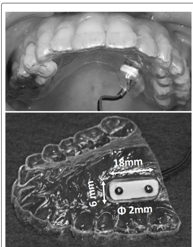
**Figure 1.** Intraoral removable device with stimulating electrodes. Participants wore the measurement apparatus, containing  $\Phi$  1-mm thermoforming discs, to ensure good contact between the oral mucosa and the stimulation electrodes.
