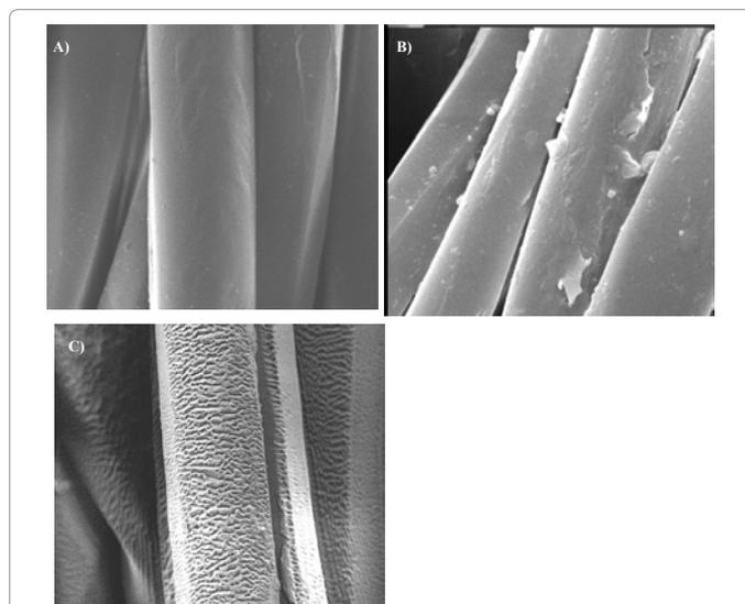
Figure 1: SEM micrographs of poly (ethylene terephthalate) fabric treated by laser and atmospheric air plasma discharge at magnification 1000: (a) untreated, (b) atmospheric air plasma treated, (c) laser treated.
