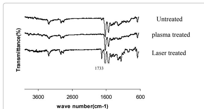
Figure 4: FTIR/ATR analysis of untreated, atmospheric air plasma and laser treated polyamide 66 fabrics.
