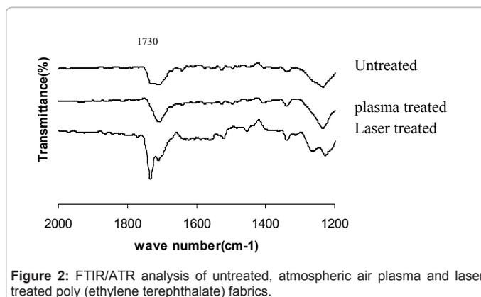
Figure 2: FTIR/ATR analysis of untreated, atmospheric air plasma and laser treated poly (ethylene terephthalate) fabrics.
