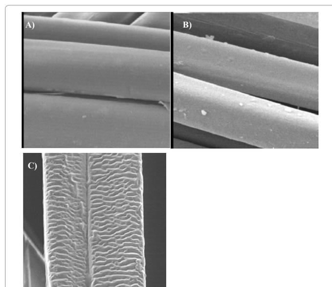
Figure 3: SEM micrographs of polyamide 66 fabric treated by laser and atmospheric air plasma discharge at magnification of 1000: (a) untreated, (b) atmospheric air plasma treated, (c) laser treated.
