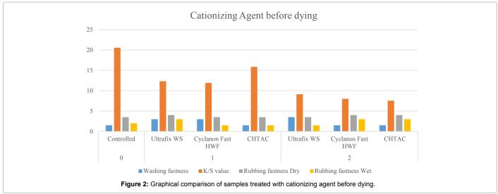
before dyeing. The use of cationizing agent increase the dye fixation by chemical reaction of positively charged substrate and negatively charged dye molecule. This method of dyeing is ecofriendly causes it is free of salt and percentage of dye in effluent is reduced.
