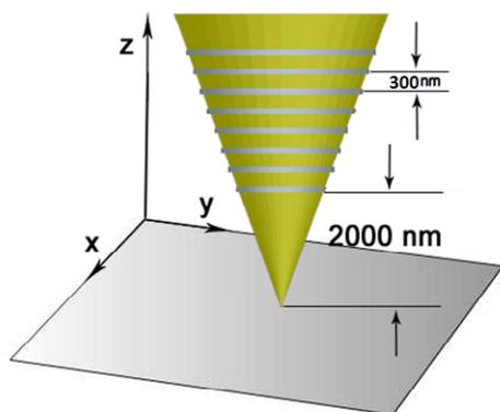
Figure 1: Considered shape for optical antenna.
