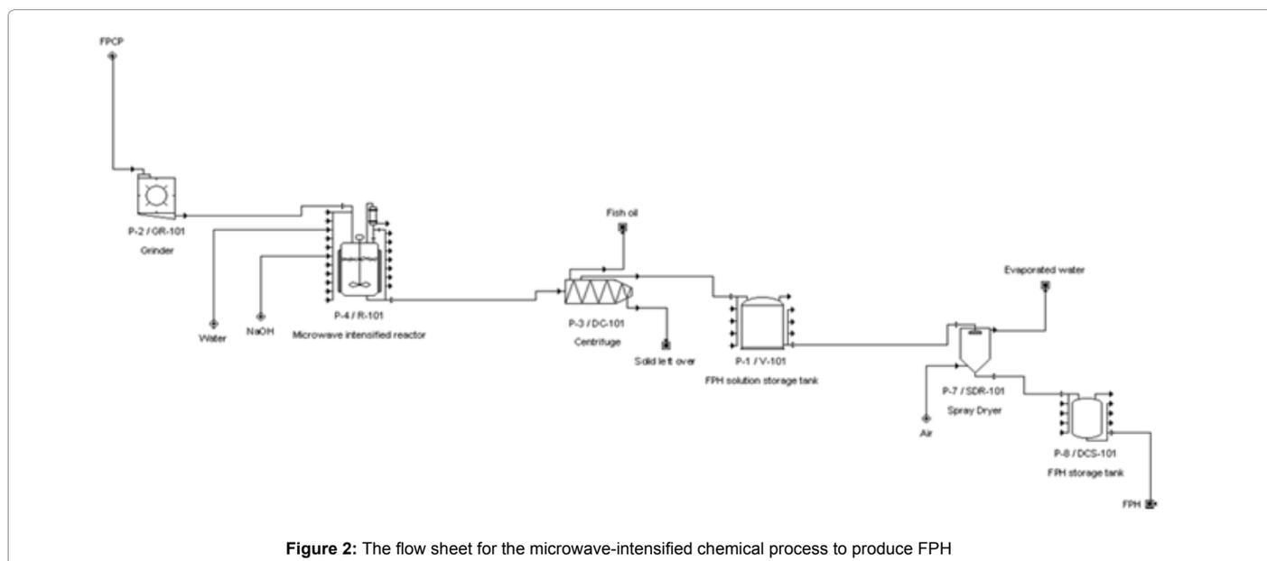
Figure 2: The flow sheet for the microwave-intensified chemical process to produce FPH
