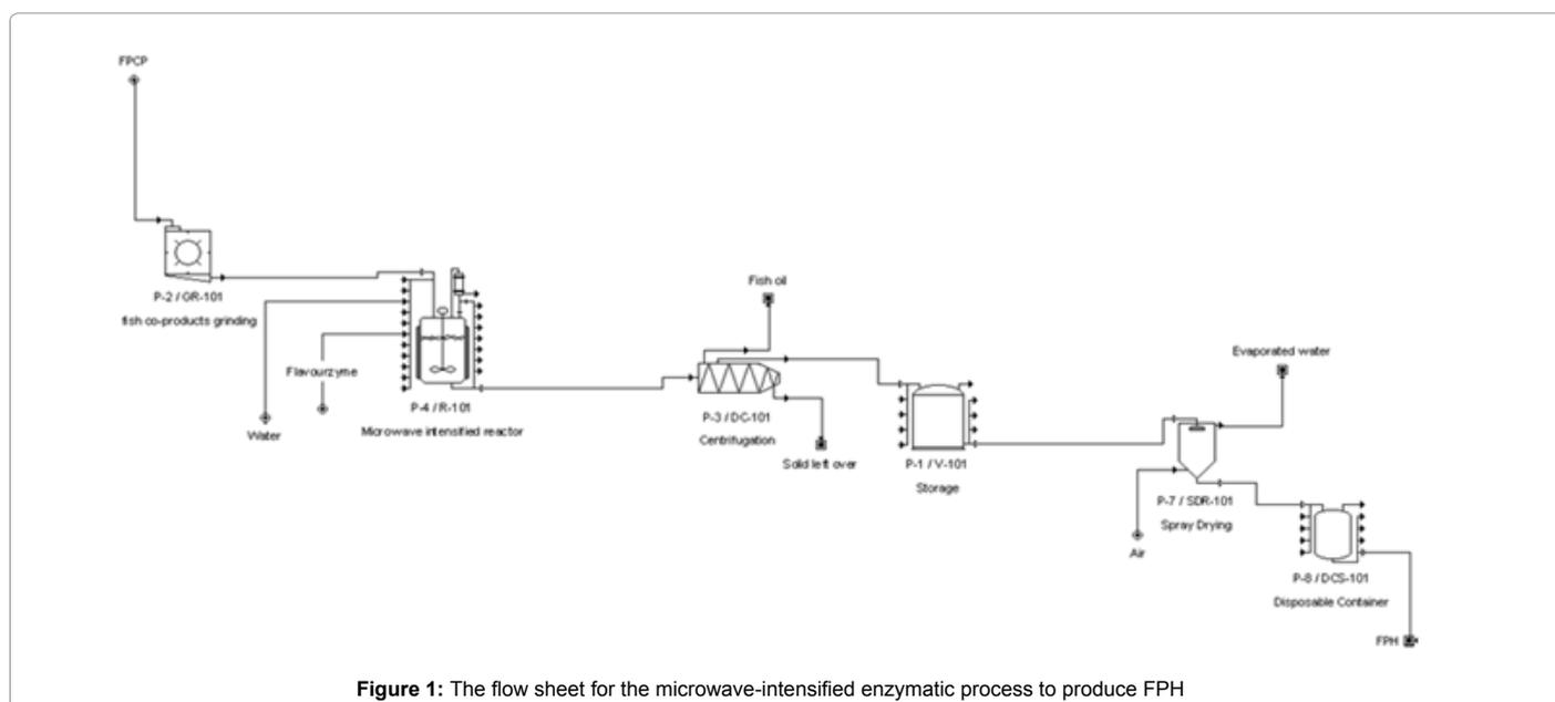
Figure 1: The flow sheet for the microwave-intensified enzymatic process to produce FPH
