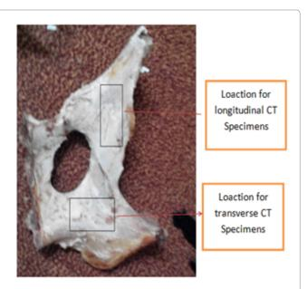
Figure 3: Location for tensile test specimens both in longitudinal and transvers direction on the bovine hip joint bone.
