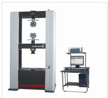
Figure 5: WDW-E-100, universal testing machine with 1000 KN loads capacity [11].
