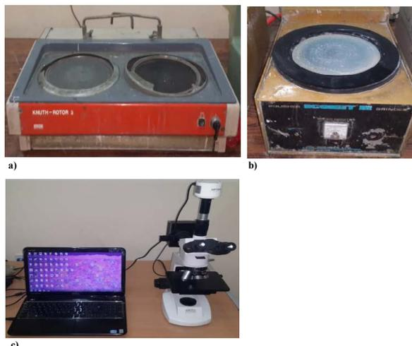
Figure 3: (a) Electric disk rotary grinding, (b) Polishing device (c) Optical microscope for microstructure observation.
