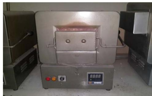
Figure 2: Electric resistance box furnace type for aging samples.
