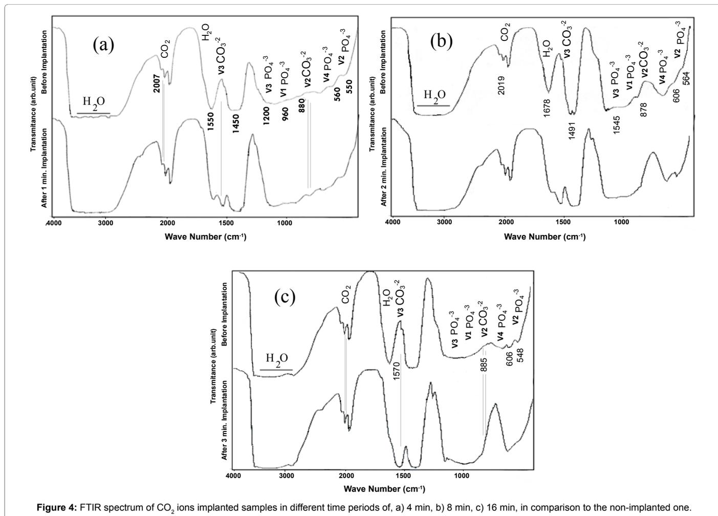
Figure 4: FTIR spectrum of CO<sub>2</sub> ions implanted samples in different time periods of, a) 4 min, b) 8 min, c) 16 min, in comparison to the non-implanted one.
