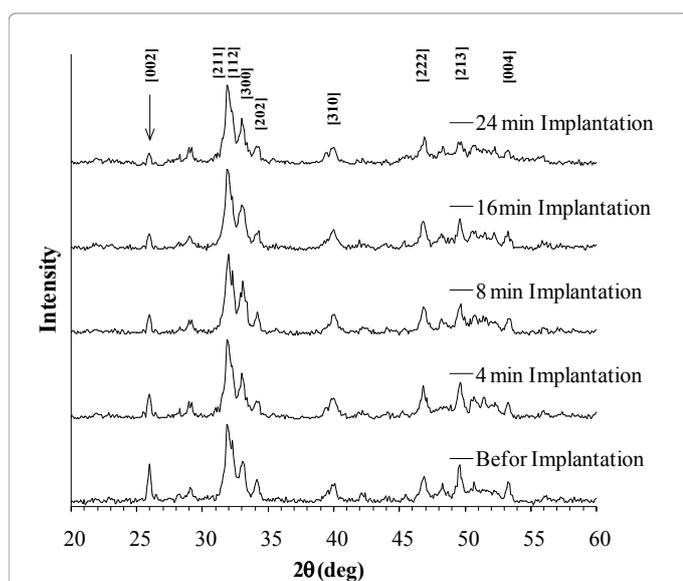
Figure 1: XRD patterns of the HAP samples implanted with CO<sub>2</sub><sup>+</sup> ions at different times in comparison to the non-implanted one (Miller indices are shown for the main peaks).
