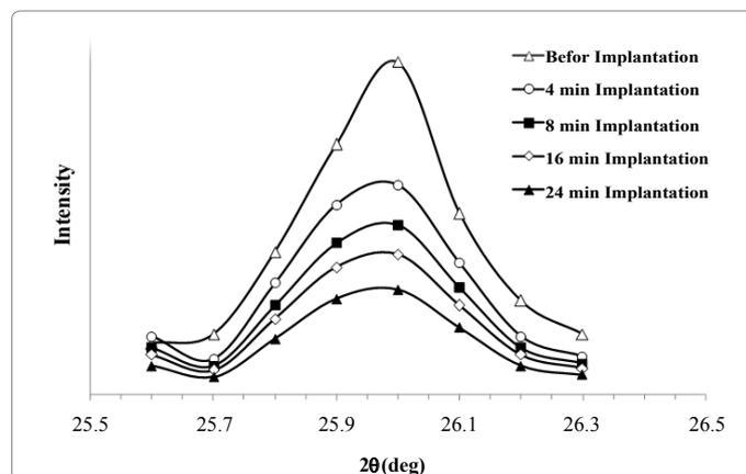
Figure 2: XRD patterns of the HAP samples implanted with CO<sub>2</sub><sup>+</sup> ions in different scales (for peak of [002]).
