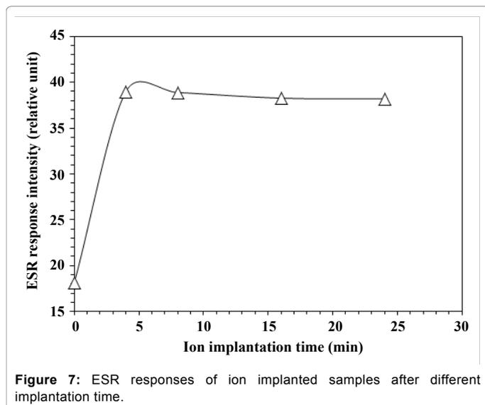
Figure 7: ESR responses of ion implanted samples after different implantation time.
