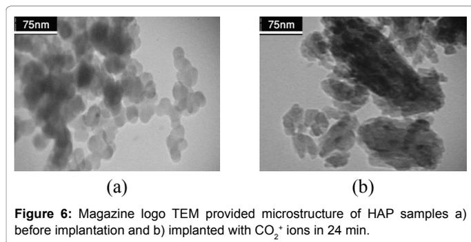
Figure 6: Magazine logo TEM provided microstructure of HAP samples a) before implantation and b) implanted with CO<sub>2</sub><sup>+</sup> ions in 24 min.
