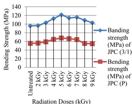
Figure 2: Bending strength of various jute reinforced polyester composites.
