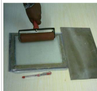
Figure 7: Hand Lay-up Technique.
