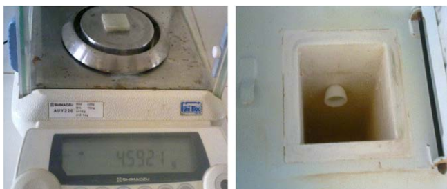
Figure 14: (a) Weight of the specimen (b) specimen in muffle furnace.
