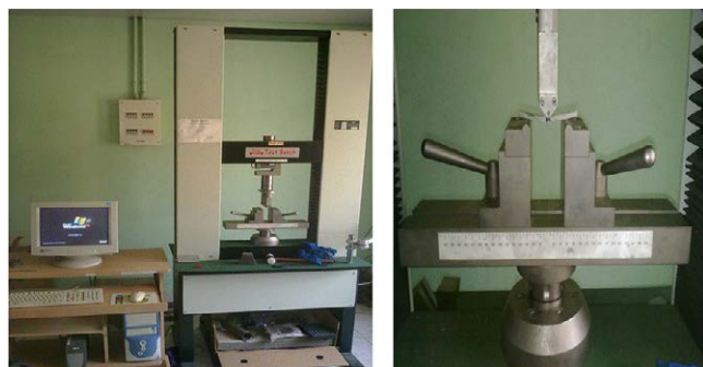
Figure 13: Universal Testing Machine for flexure test.
