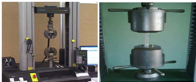
Figure 12: Universal Testing Machine for Tensile test.
