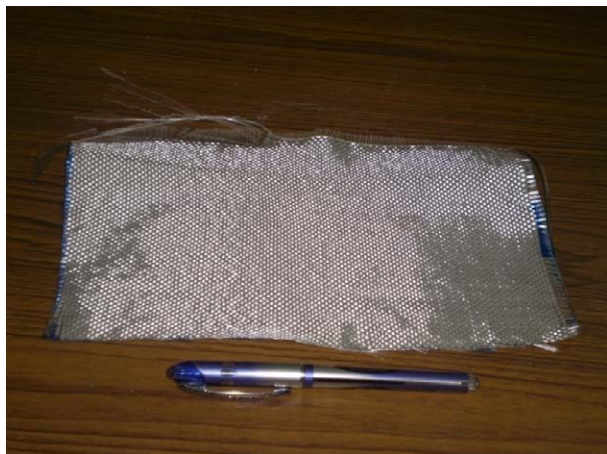
Figure 4: Bi directional s-glass woven fibre.
