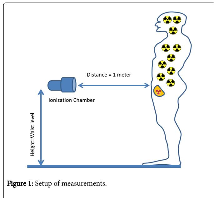
**Figure 1:** Setup of measurements.
