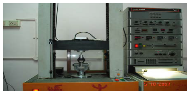
Figure 4: Test set-up for pull-out test.
