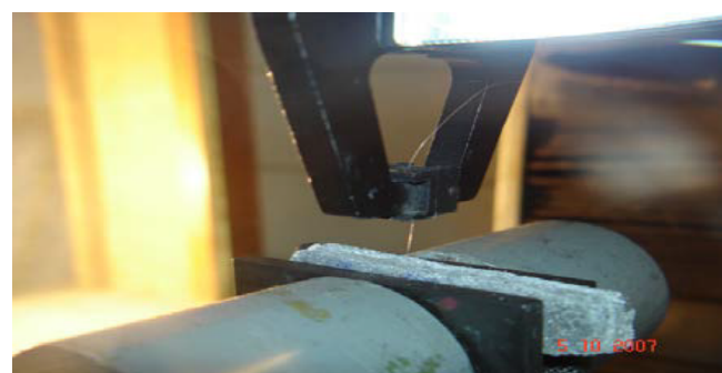
Figure 5: Grips for fiber and specimen.
