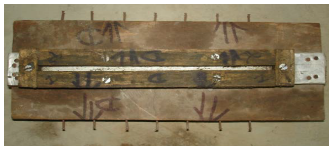
Figure 3: Pull out mould for 6 mm thickness.
