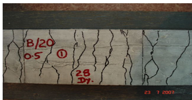
Figure 7: Multiple cracks in 20 mm beam.
