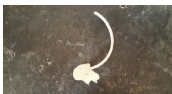
Figure 5: Fluidity spiral length 307mm at a pressure of 0 MPa.
