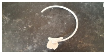
Figure 6: Fluidity spiral length 415 mm at a pressure of 30 MPa.
