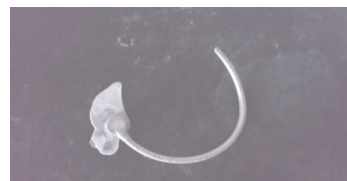
Figure 7: Fluidity spiral length 359 mm at a pressure of 60 MPa.
