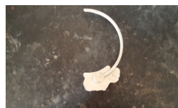
Figure 8: Fluidity spiral length 316 mm at a pressure of 90 MPa.
