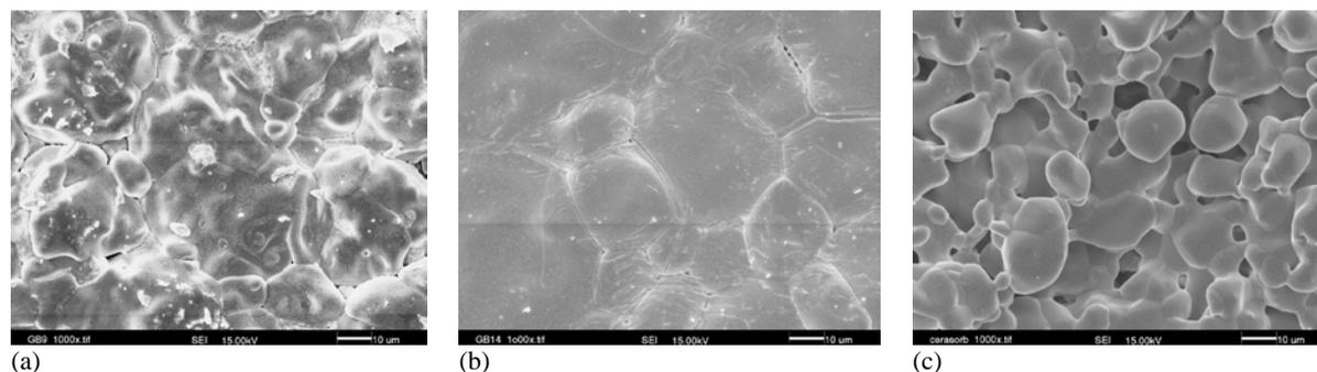
**Figure 2:** Scanning electron micrographs of the various calcium phosphate specimens after fabrication of the disc-shaped substrata: (a) GB9, (b) GB14, and (c)  $\beta$ -TCP (original magnification 1000x).
