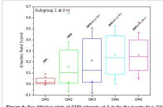
Figure 1: Box-Whisker plots of EMR intensity at 0 m for the twenty-four (24) mobile devices of Subgroup 1 at the five different operation modes (OM1 to OM5).
