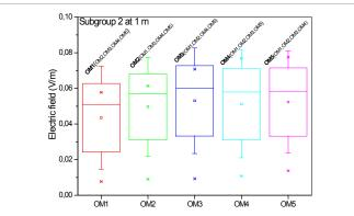
Figure 5: Box-Whisker plots of EMR intensity at 1 m for the nine (9) mobile devices of Subgroup 2 at the five different operation modes (OM1 to OM5).
