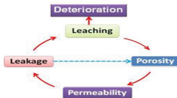
Figure 1: Cyclic process for leaching deterioration of concrete.
