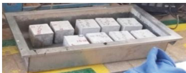
Figure 7: Specimens inside equipment to allow water absorption.
