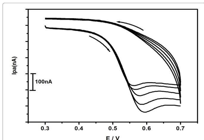
Figure 8: Cyclic voltammograms of different concentrations for BPA at TBMCPCE.
