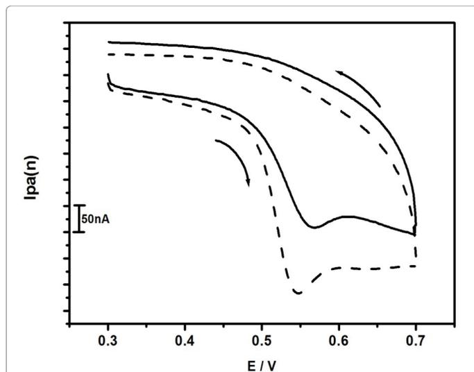
Figure 4: Cyclic voltammograms of 5 nM Bisphenol-A at bare carbon paste electrode (solid line) and modified carbon paste electrode TBMCE (dashed line) with scan rate of 50mVs<sup>-1</sup>.
