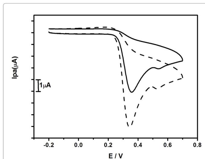
Figure 11: Cyclic voltammograms of 7nM BPA and 1mMUA at TBMCPCE.
