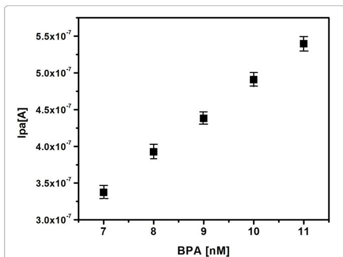
Figure 9: Plot of anodic peak current versus concentration of BPA.
