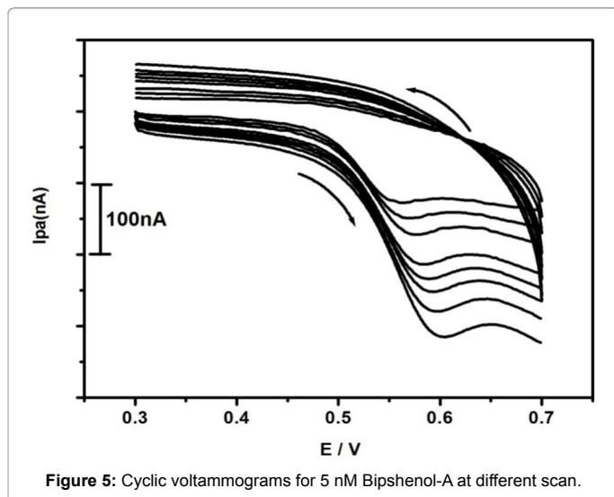
Figure 5: Cyclic voltammograms for 5 nM Bipshenol-A at different scan.
