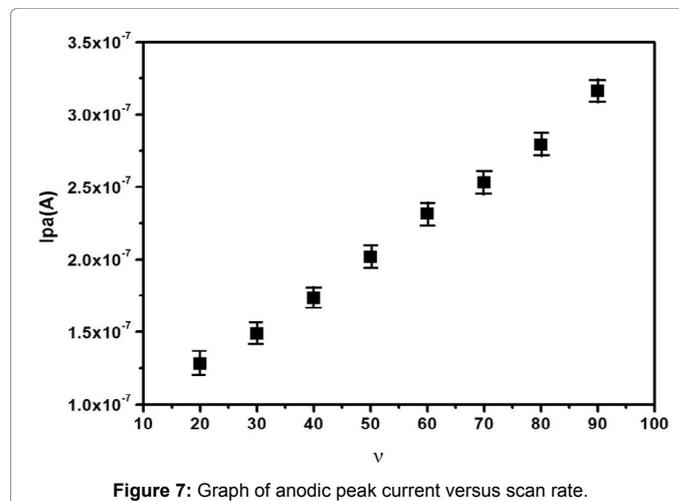
Figure 7: Graph of anodic peak current versus scan rate.
