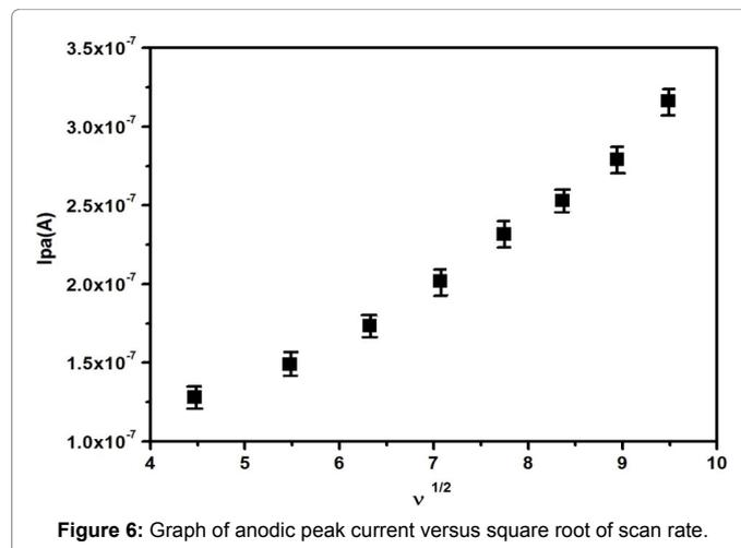
Figure 6: Graph of anodic peak current versus square root of scan rate.
