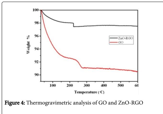
**Figure 4:** Thermogravimetric analysis of GO and ZnO-RGO
