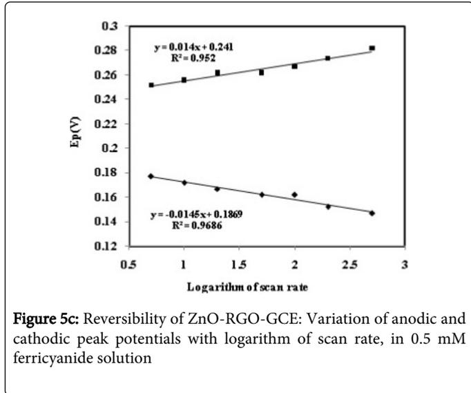
**Figure 5c:** Reversibility of ZnO-RGO-GCE: Variation of anodic and cathodic peak potentials with logarithm of scan rate, in 0.5 mM ferricyanide solution
