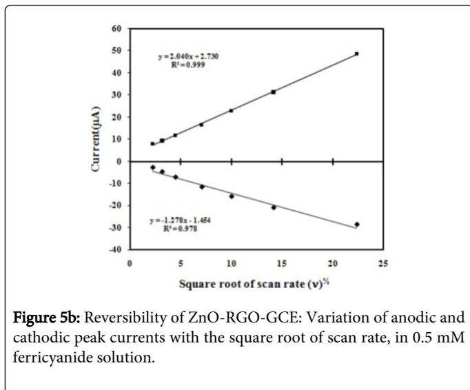
**Figure 5b:** Reversibility of ZnO-RGO-GCE: Variation of anodic and cathodic peak currents with the square root of scan rate, in 0.5 mM ferricyanide solution.
