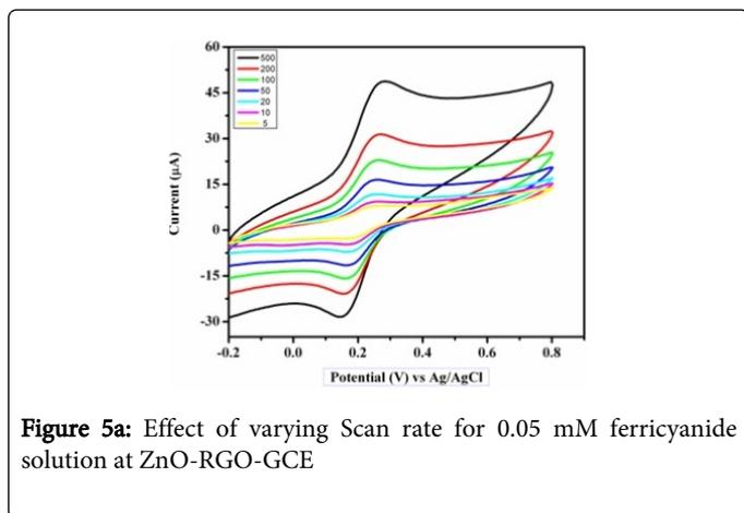
**Figure 5a:** Effect of varying Scan rate for 0.05 mM ferricyanide solution at ZnO-RGO-GCE
