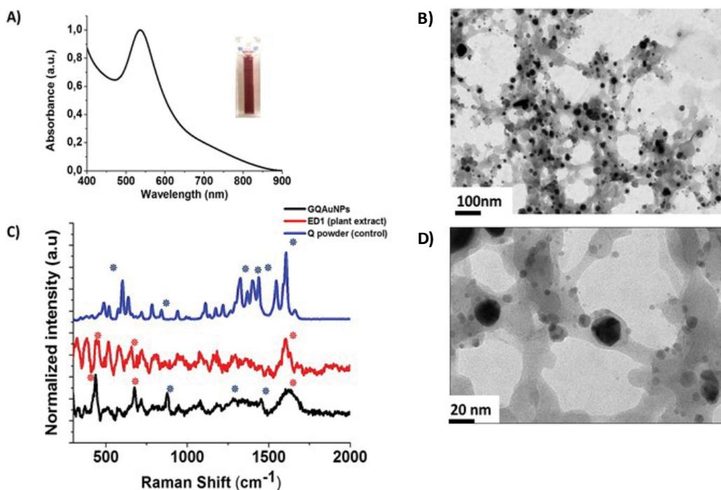
**Figure 3:** (A) Normalized UV-Vis absorption, (B) TEM and High TEM magnification (D) images, (C) normalized Raman spectra of the selected GQAuNPs (QTSK1) compared to TSK1 extract plant and free Quercetin (Q) as control. (B, D) Scale bars: 100 nm and 20 nm. (C) Experimental conditions:  $\lambda_{exc} = 785$  nm; laser power 22 mW; accumulation time 100 s.
