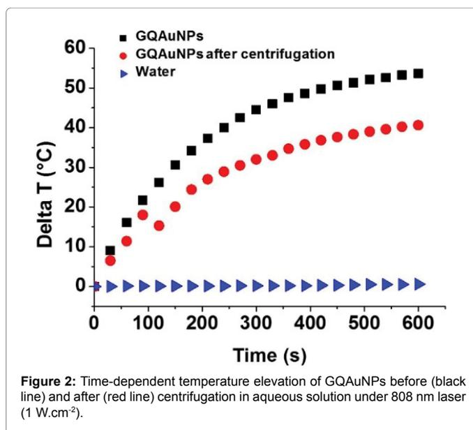
**Figure 2:** Time-dependent temperature elevation of GQAuNPs before (black line) and after (red line) centrifugation in aqueous solution under 808 nm laser ( $1 \text{ W.cm}^{-2}$ ).
