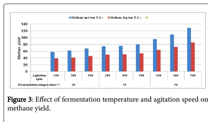
Figure 3: Effect of fermentation temperature and agitation speed on methane yield.
