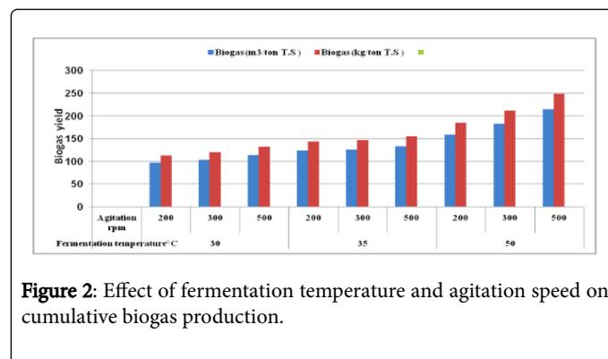
Figure 2: Effect of fermentation temperature and agitation speed on cumulative biogas production.
