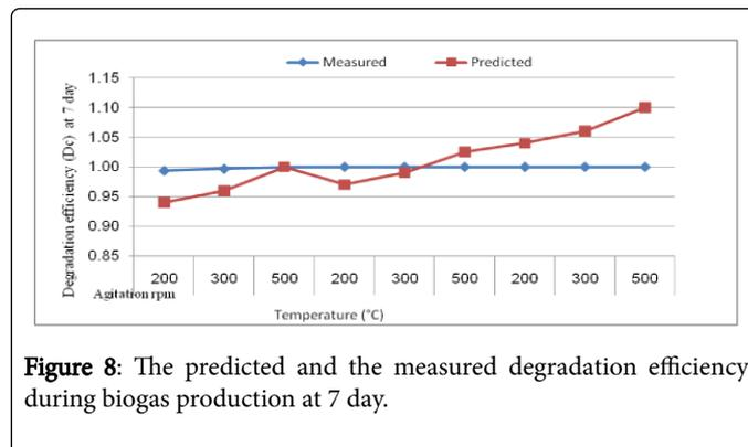
Figure 8: The predicted and the measured degradation efficiency during biogas production at 7 day.
