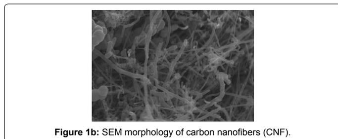
Figure 1b: SEM morphology of carbon nanofibers (CNF).
