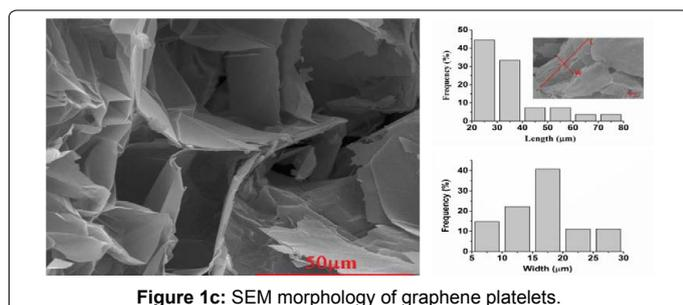
Figure 1c: SEM morphology of graphene platelets.
