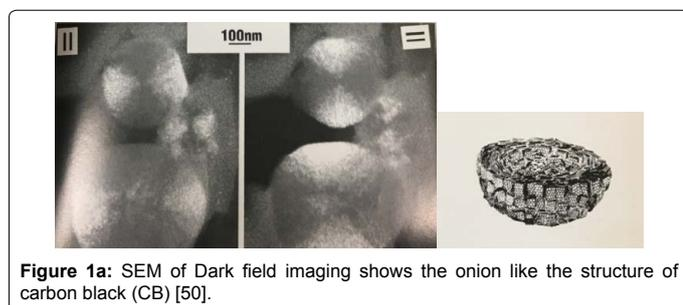
Figure 1a: SEM of Dark field imaging shows the onion like the structure of carbon black (CB) [50].
