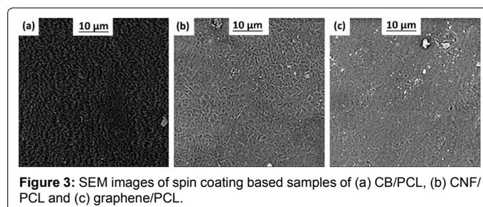
Figure 3: SEM images of spin coating based samples of (a) CB/PCL, (b) CNF/PCL and (c) graphene/PCL.
