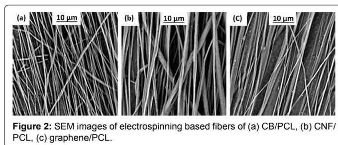
Figure 2: SEM images of electrospinning based fibers of (a) CB/PCL, (b) CNF/PCL, (c) graphene/PCL.
