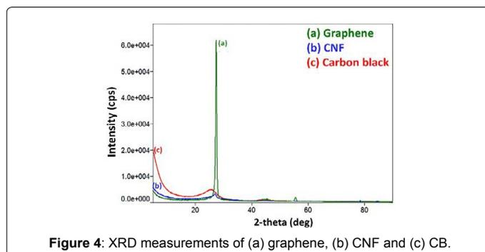
Figure 4: XRD measurements of (a) graphene, (b) CNF and (c) CB.
