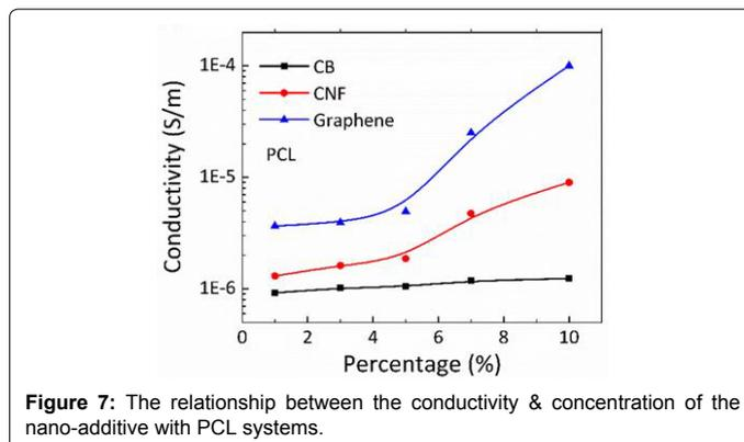
**Figure 7:** The relationship between the conductivity & concentration of the nano-additive with PCL systems.
