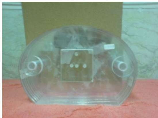
Figure 4: Phantom for Monte Carlo validation.
