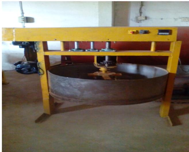
Figure 1: Electro-mechanical gari roaster
